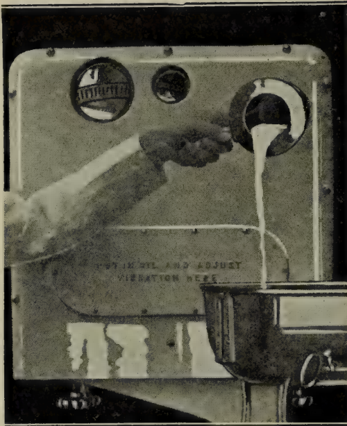
Fig. 108. Emptying Overrun Cup Into Freezer Hopper.
